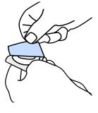
**Step 3)** Place one side of the transfer tape onto the surface, and press it down with the vinyl applicator.
