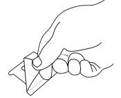
**Step 6)** Beginning in a corner, slowly peel away the transfer tape at a 45 degree angle.
